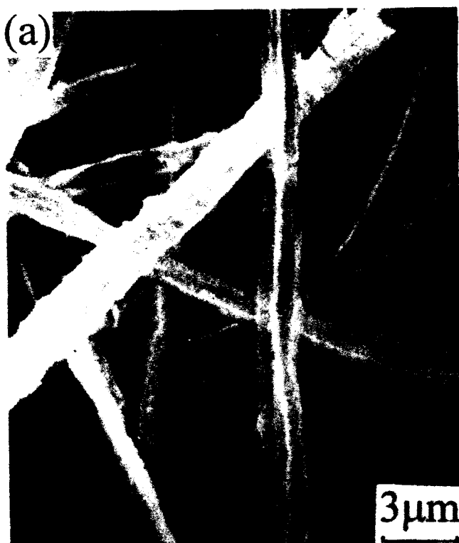
Fig. 3. Scanning electron microscopy photographs of Ni fibers of diam 2 μm at two magnifications.
